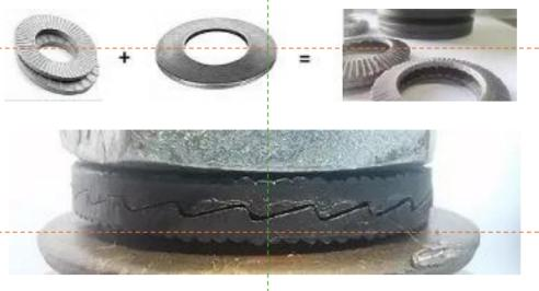
When the fasener is tightened the CAMS lock and he GRIPS on the outer surfaces embed themselves into the fastener nut and the clamped part, leaving impressions on both. Because the gradient of of the wedges is greaer than the size of the fasteners pitch, any rotational movement results in tightening of the wedges and an increase in preload, thus securing the assembly.
